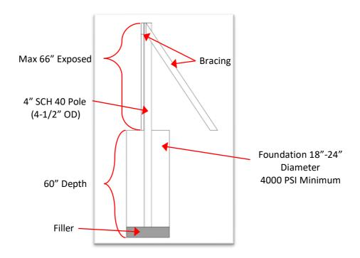
NOTE: The pole must be installed perfectly vertical and should be braced during pouring and setting of the foundation. Allow the concrete to set for at least 24 hours before continuing with the installation of the mount.
