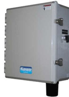
Optional UL Approved, 208/240V Power Control Panel complete with 30ma Protected Ground Fault Interrupter, 24 Hour Mechanical Timer, Surge Protector, and Hand-Off-Auto switch. NEMA Type 4x/3r non-metallic enclosure.
