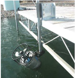
Kasco's heavy duty dock or piling mount is made from corrosion protected steel and stainless steel. This dock mount can be used with any of our de-icer units. Users supply their own 10 foot 1" O.D. pipe. Includes a Qwiklock handle for easy installation and adjustments
