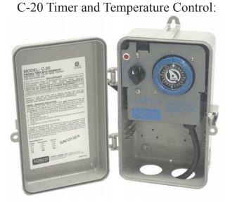
Kasco's C-20 further maximizes energy conservation from the C-10 with the added timer feature. The C-20 will only operate your De-icer when both the timer and thermostat are activated. Horizontal Float:
