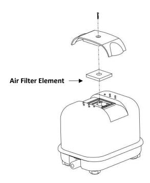
Replacement air filter elements are readily available. Contact your local Kasco distributor and ask for the appropriate Replacement Air Filter Element per the list below.
